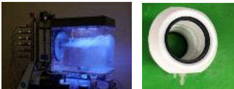
Fig. 1 Picture of online mechanical chemical cleaning system (Left) and cleaning column(Right)
